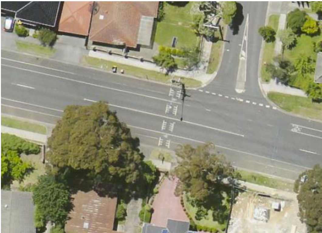
FIGURE 12: EXAMPLE OF SPEED CUSHION TREATMENTS – HAWTHORN ROAD, BURWOOD EAST
