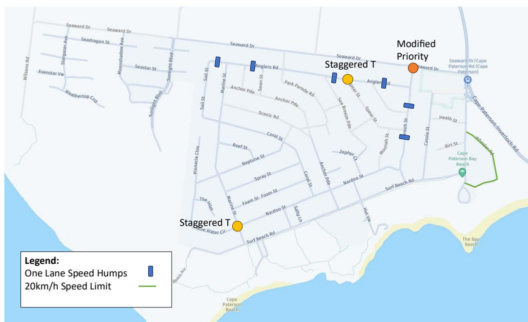
FIGURE 5: EXISTING LOCAL STREET TRAFFIC MANAGEMENT TREATMENTS
